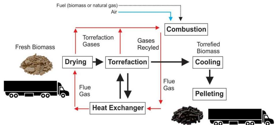
**Figure 1.** Torrefied pellets processing flowchart [10].
