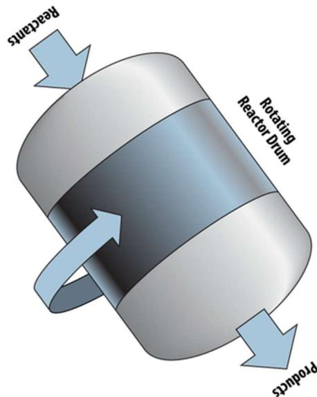
**Figure 6.** Rotary drum reactor for biomass torrefaction [60].
