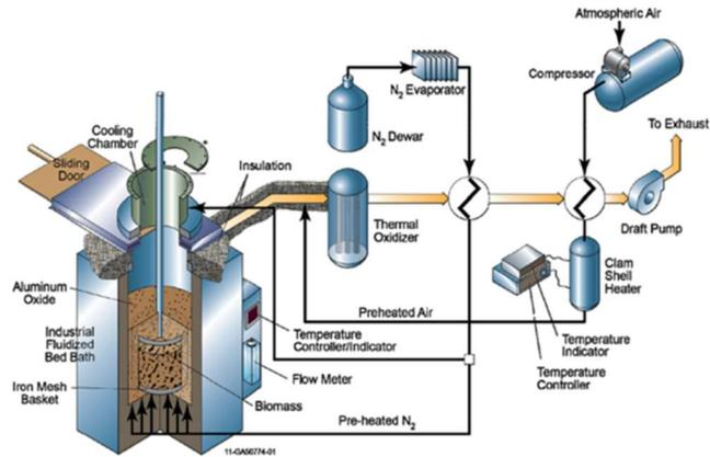
**Figure 5.** Fixed bed reactor for biomass torrefaction [76].
