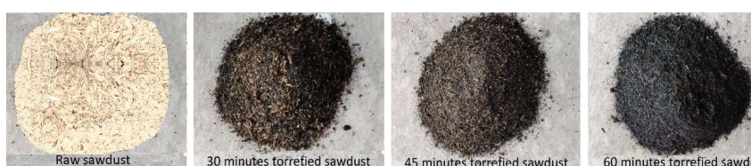
Figure 9. Samples of untreated and torrefied sawdust produced at 30, 45, and 60 min [12].
