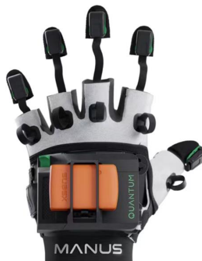
Figure 2. Hand motion tracking system.
