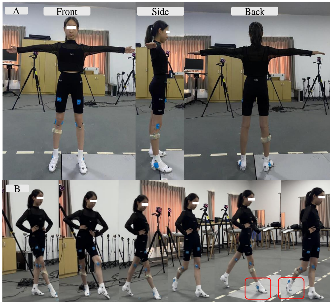
Figure 1. (A) Illustration of placing reflex markers on human skeletal markers and EMG electrodes on human lower limbs; (B) illustration of the Rumba Walk test procedure.
