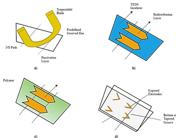
**Figure 6.** Methodology of the silicon groove technology. (a) Stage 1; (b) Stage 2; (c) Stage 3; (d) Stage 4.
