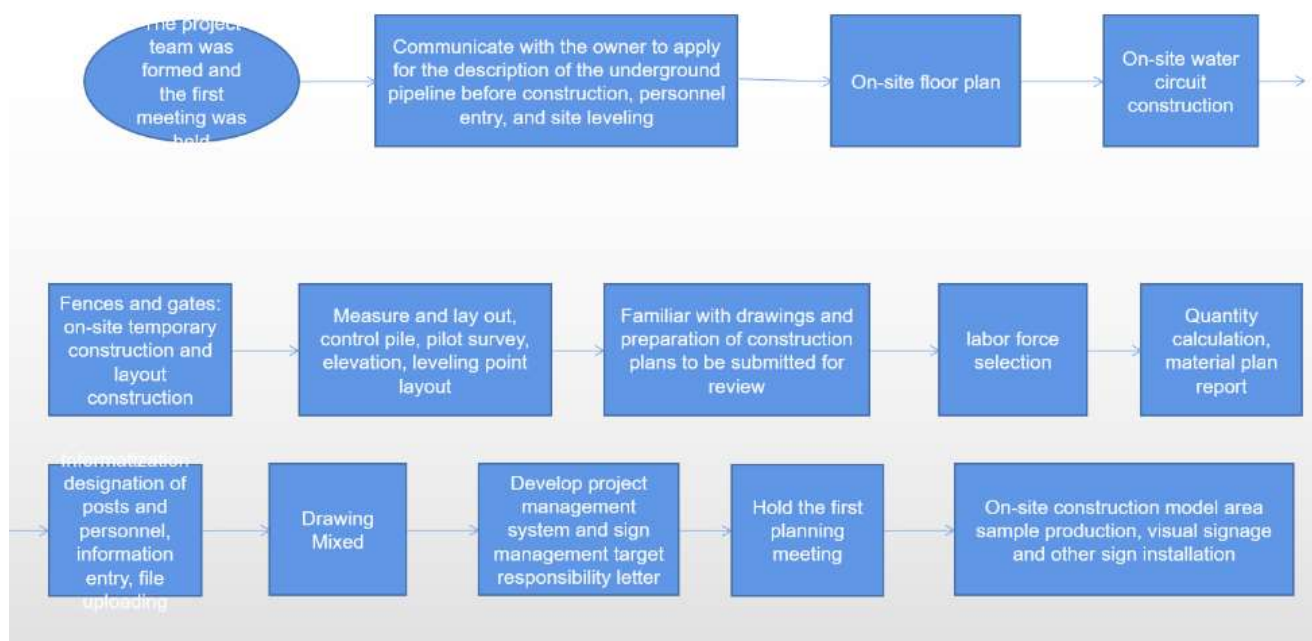
Figure 8. Construction steps of high-rise residential buildings.
